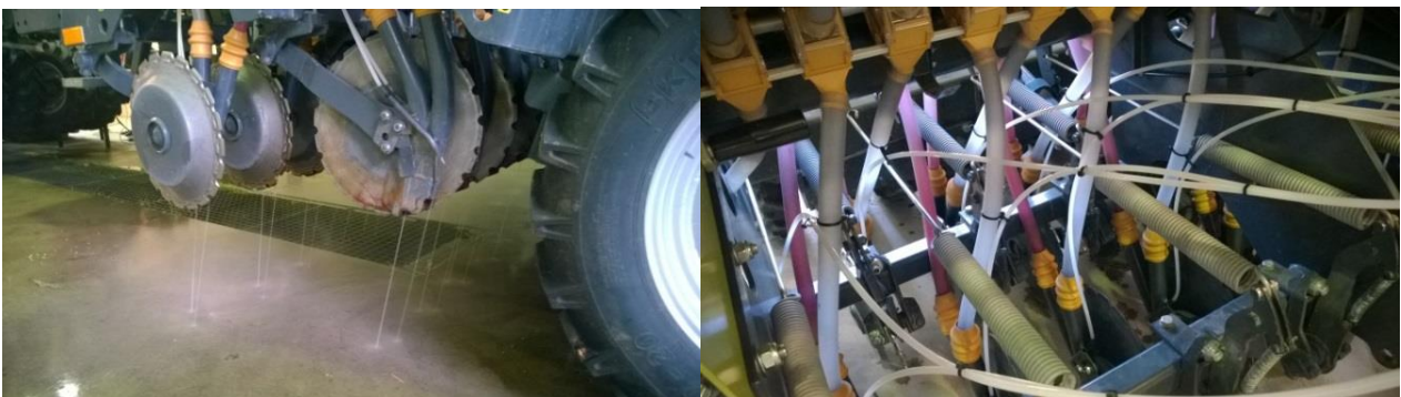
Figure 6. Additional hoses for liquid fertilizers (thin white hoses) assembled to the combined seed drill (left). Special disc coulters where liquid fertilizer hoses are attached to, enabling placement application of additional two liquid fertilisers (right).
