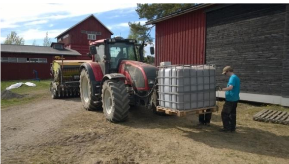
Figure 12. Mounting the Bio-Kali tank to the front of the tractor and checking the automation settings in the task controller before starting the actual field work.
