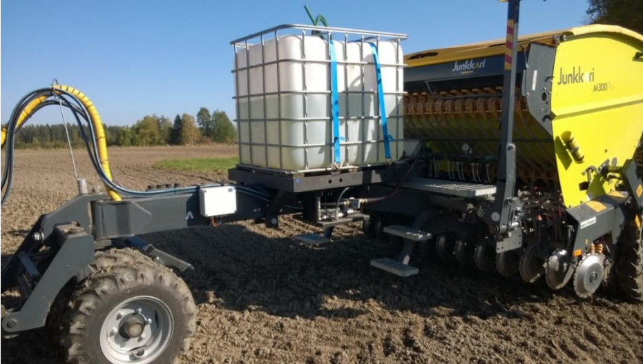
Figure 11. Recycled liquid AMS tank, pump (under the tank) and the ISOBUS controller (white box) were placed on the pulling shaft of the combined seed-driller.
