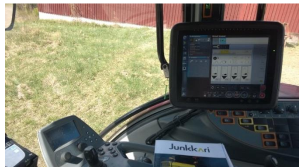
Figure 12. Mounting the Bio-Kali tank to the front of the tractor and checking the automation settings in the task controller before starting the actual field work.
