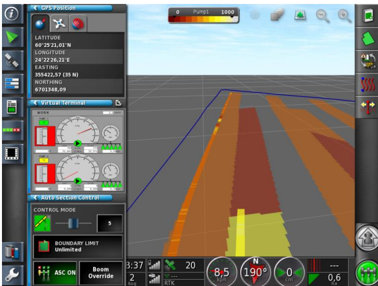
Figure 8. ISOBUS compatible Valtra C3000 Task controller as a user interface for the machine combination.
