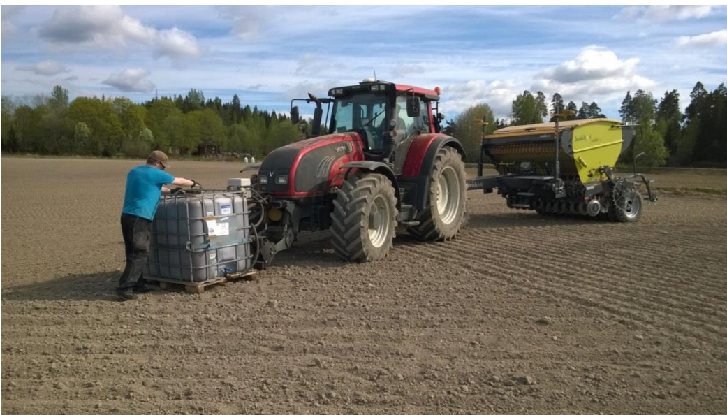
Figure 10. The machinery combination in the first demonstration: ISOBUS equipped tractor, precision combined seed driller and application system for recycled liquid fertilizer (Bio-Kali).
