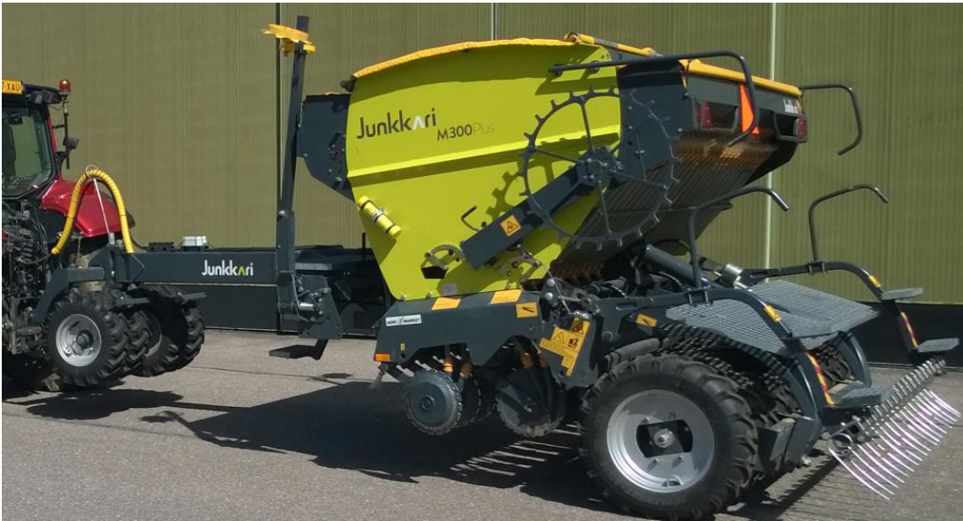
Figure 5. Junkkari M300 Plus combined seed drill with four site-specifically controllable containers; 1 for cereal seed, 1 for granule fertilizer, 2 for small seed or granule micronutrients.
